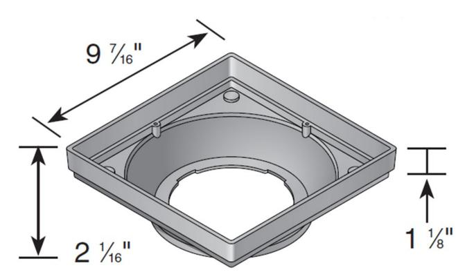
Part #: 930 Material: (HIPS) High Impact Polystyrene Color: Black Fits: 3" and 4" Sch. 40 pipe, 3", 4", 6" and 8" sewer, drain , corrugated and triple wall pipe. Requires NDS Universal Outlet #1243, #1245, #1266, or #1889. Use with 9" x 9" Grates Weight Per Each: 0.813 lbs. UV inhibitor
